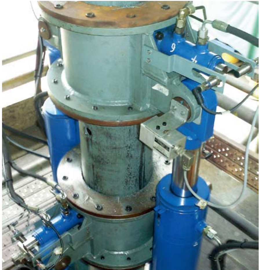
Testing of KOMtech and OTD's hydraulic jacking system prototype was conducted at Keppel FELS
