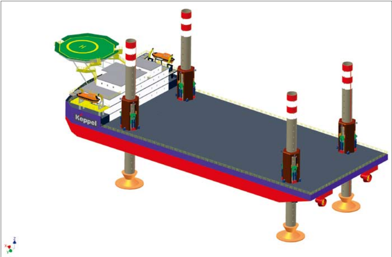
Overview of a vessel installed with the OTD hydraulic jacking system
